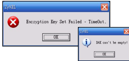
Figure 45 Incorrect DAK or No DAK
